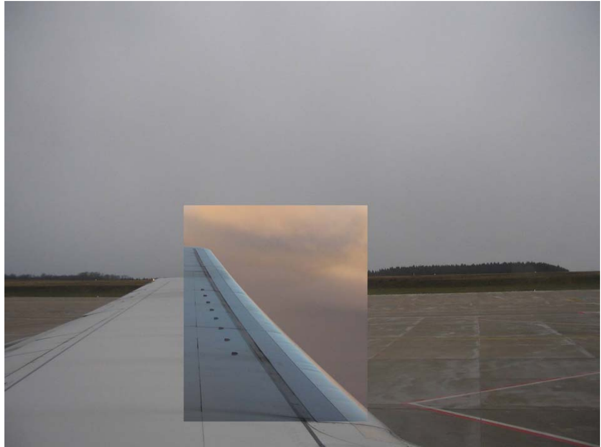
Boeing 737-800 at ground and in cruise ( Ma = 0.76 )
