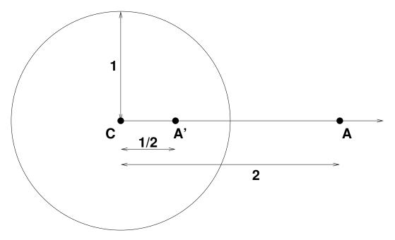
9. Given a circle c with centre C and a point A, construct the image of A' under the inversion on the circle c.
