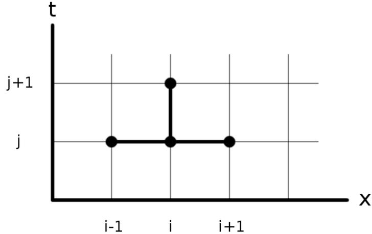
FIGURE 5. Stencil of the Lax-Wendroff-scheme in example 2.15
